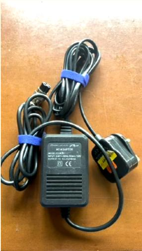
The power supply is a transformer with a stated output of 19.5V x2 at 200mA.
